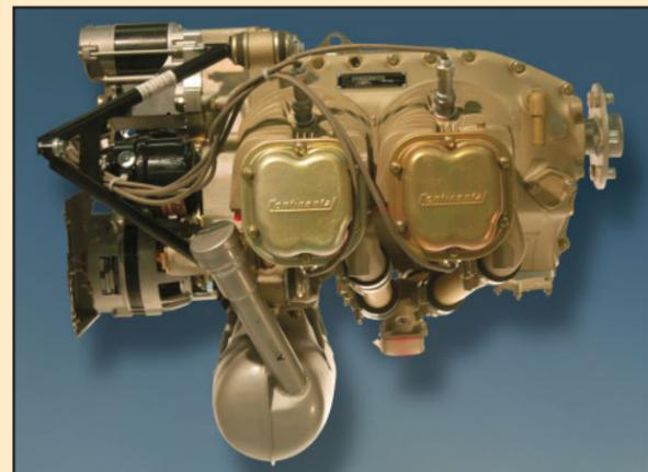
*The Continental O-200 four-cylinder, 100 hp engine is as legendary as the Cub itself. It has provided countless hours of reliable operation in a wide variety of aircraft applications. Parts and maintenance are readily available at virtually any maintenance facility.*
